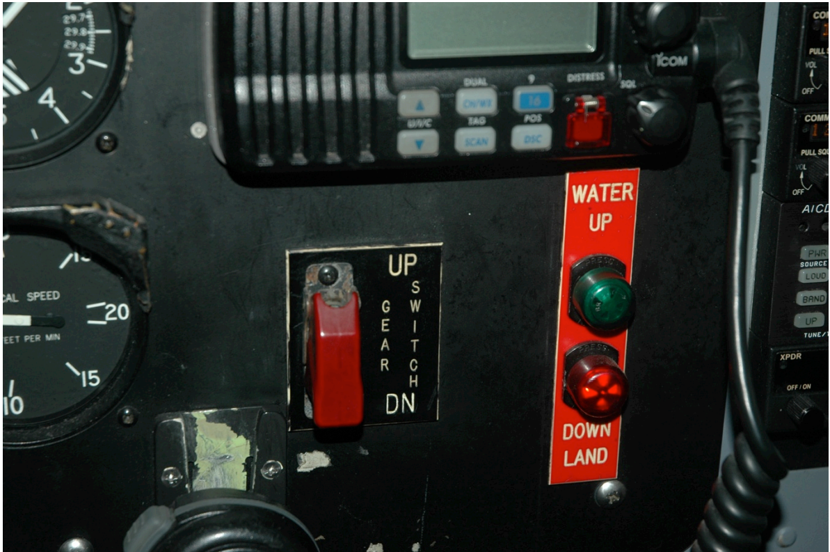
Figure 1 Gear position lights that have been modified to indicate the gear-down position with a red light. This calls attention to the fact that that 'wheels-down' is an inherently hazardous configuration.
