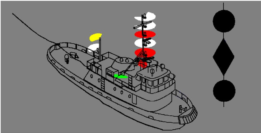
Vessel engaged in towing operation which severely restricts towing vessel and her tow in their ability to deviate from their course—length of tow does not exceed 200 meters; towing vessel less than 50 meters in length. Same for International.
