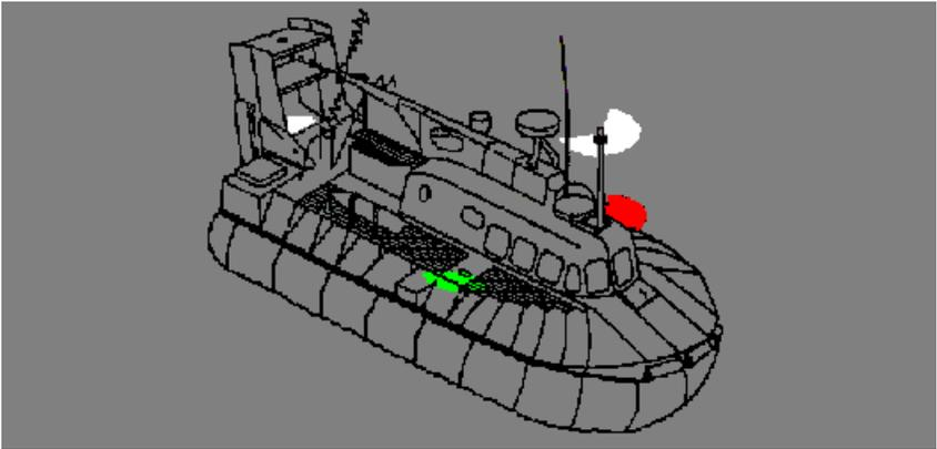
Air-cushion vessel when operating in the displacement mode—
