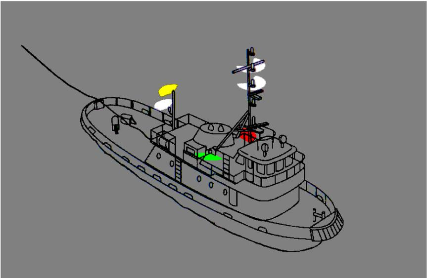
Power-driven vessel towing astern—towing vessel less than 50 meters in length; length of tow 200 meters or less. Same for International.
