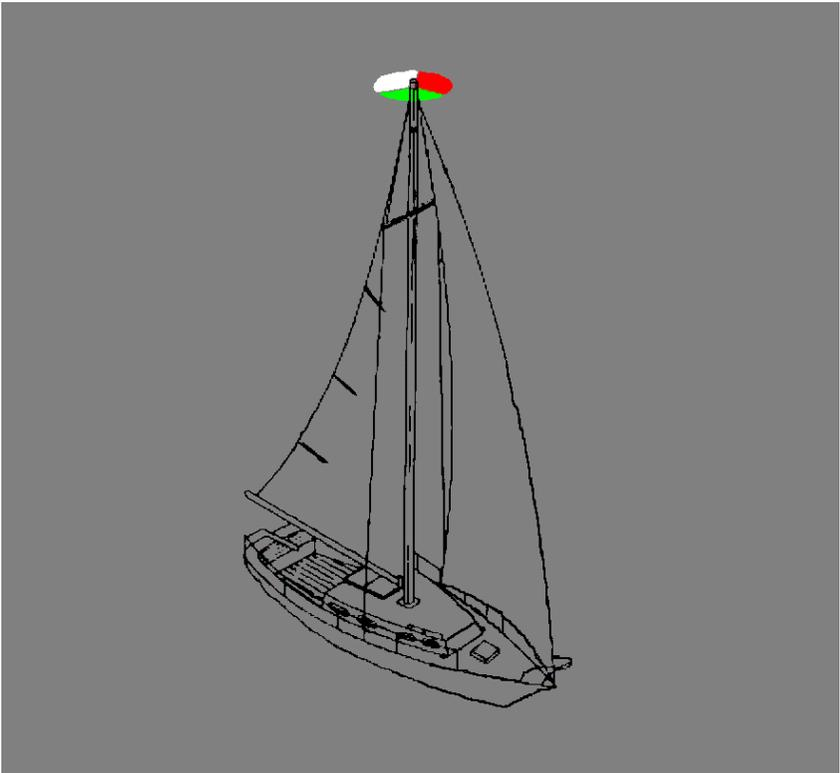
Sailing vessel underway—less than 20 meters in length.
