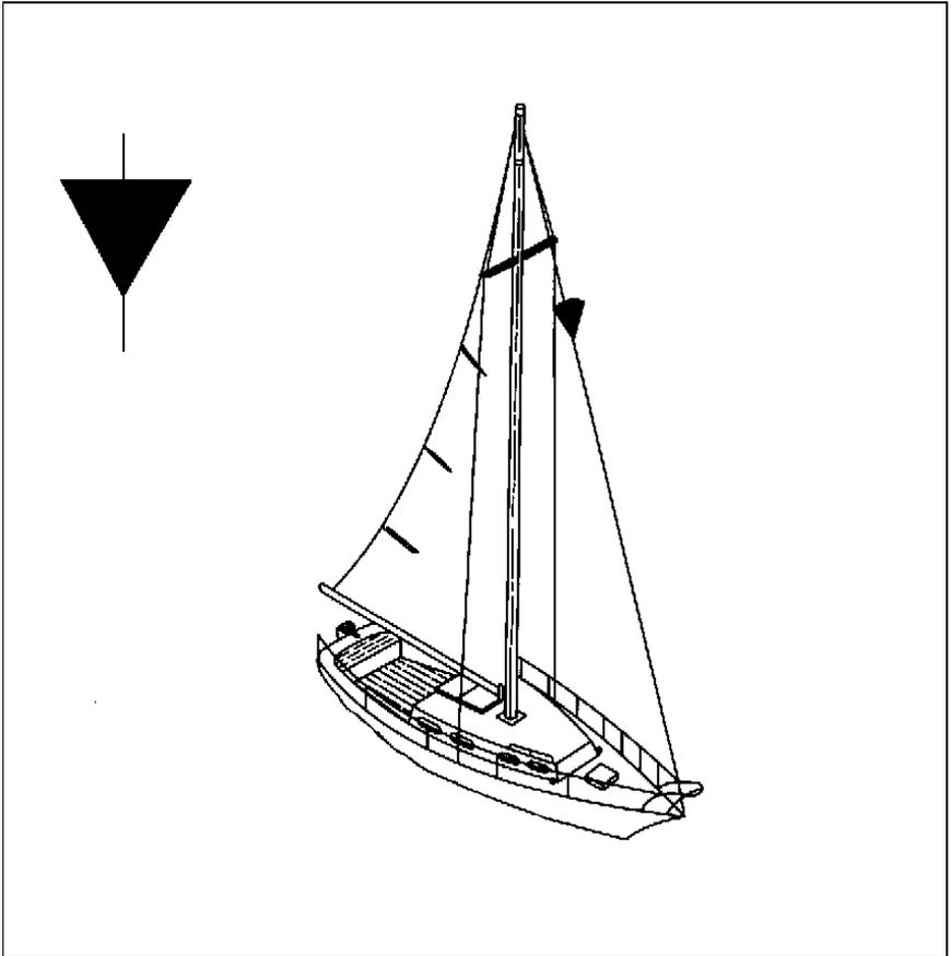
Vessel proceeding under sail when also being propelled by machinery.
