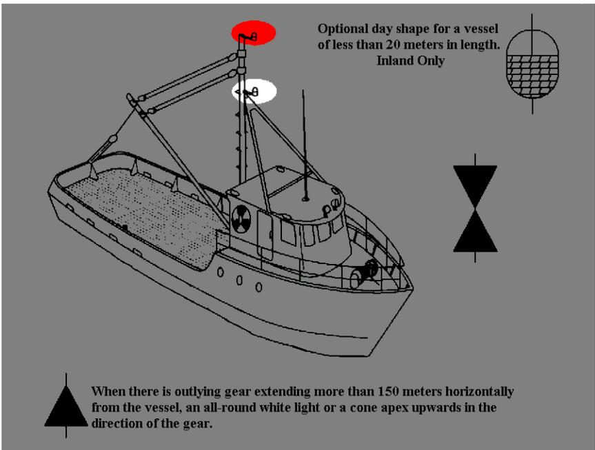
Vessel engaged in fishing other than trawling—not making way.
