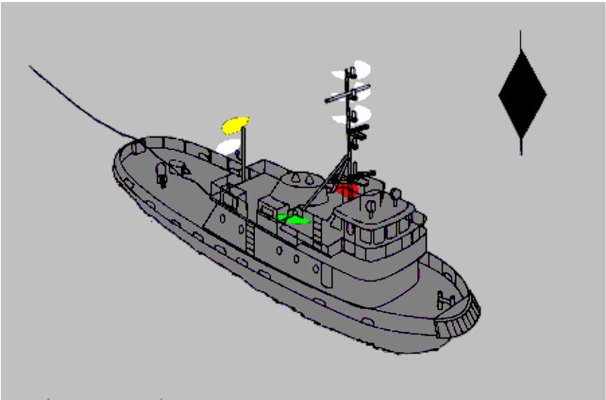
Power-driven vessel towing astern—towing vessel less than 50 meters in length; length of tow exceeds 200 meters.
